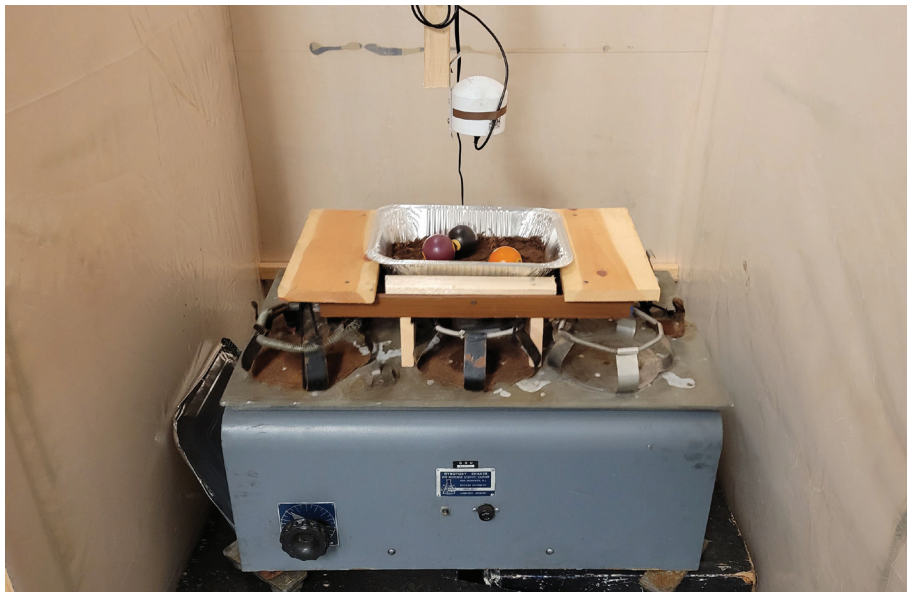
Materials were dried and tested for particulates 2.5 microns or smaller (PM 2.5 ) in a testing chamber with MERV 13 filtration. Each material was agitated as the surrounding air was tested for one hour. | Images courtesy of Brad Steinmetz.
